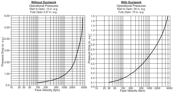
Typical performance for Model PRI4 backdraft damper size tested 42"W x 42"H furnished with counterweight to assist opening.
